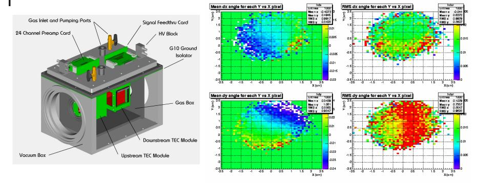
The TEC (time expansion chamber) is a transverse drift chamber operating at 0.08 bar, separated from beam vacuum by 6  $\mu$ m Mylar windows. It has two modules, one for x and one for y.
