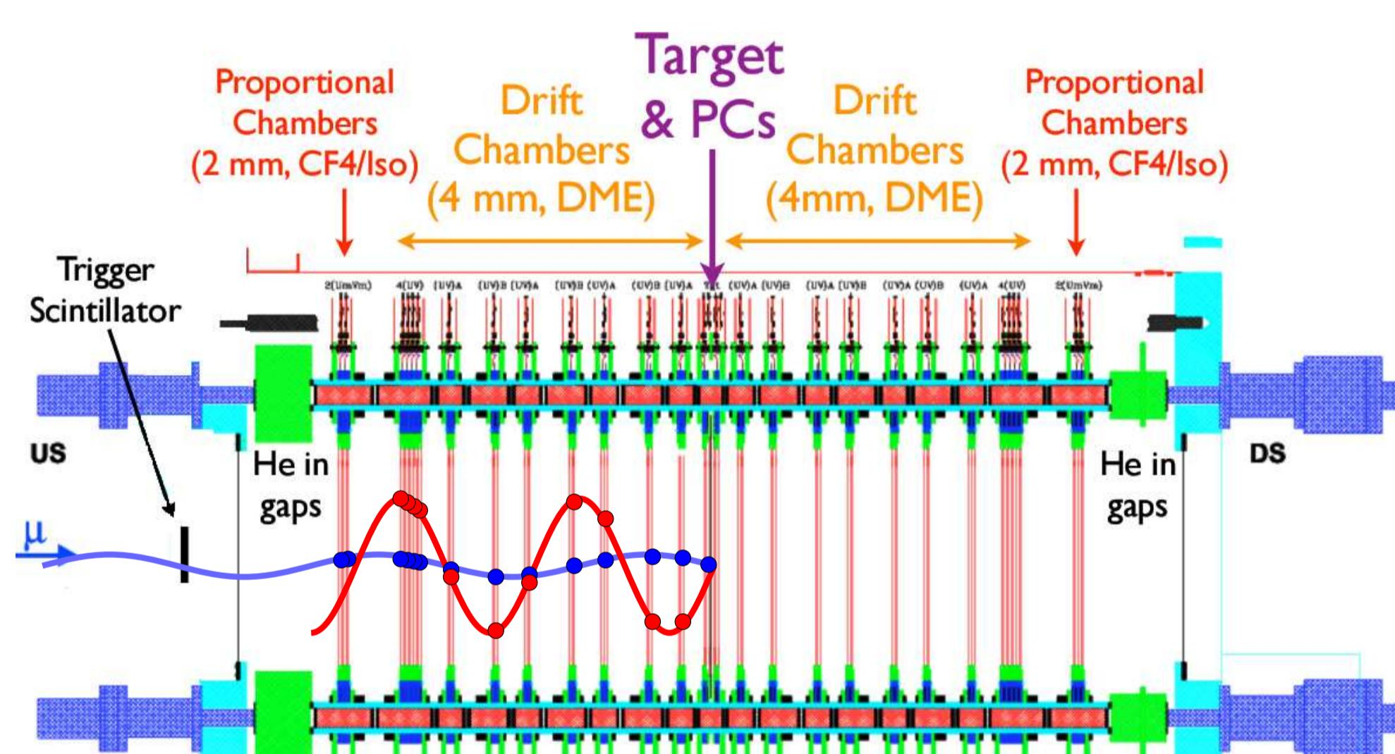
A low mass, high precision spectrometer inside 2T magnetic field measures **positrons ( $e^+$ )** and **muons ( $\mu^+$ )**.
